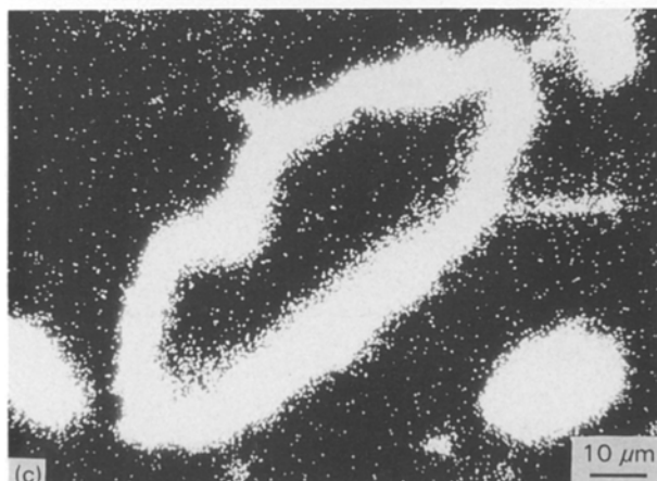
Figure 8 EPMA micrographs showing the onset of reaction of a carbon particle with the titanium of the melt: (a) SEI picture, (b) C X-ray mapping, and (c) Ti X-ray mapping.
