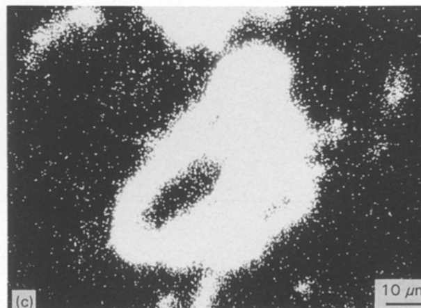
Figure 9 EPMA micrographs showing further reaction through penetration of the carbon particle by the melt: (a) SEI picture, (b) C X-ray mapping, and (c) Ti X-ray mapping.
